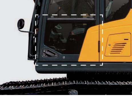
The auto safety lock feature prevents unintentional ignition. While the auto safety lock is activated, the excavator is not controlled by the RCV lever.
