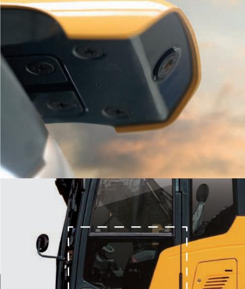
The All-Around View Monitoring (AAVM) camera system gives you a 360° overview of your immediate working environment. It also includes Intelligent Moving Object Detection (IMOD) technology that senses and warns you when people or objects come within five metres of the machine.
