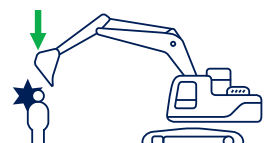
Excavator is not controlled by RCV lever and prevents unintended operation
