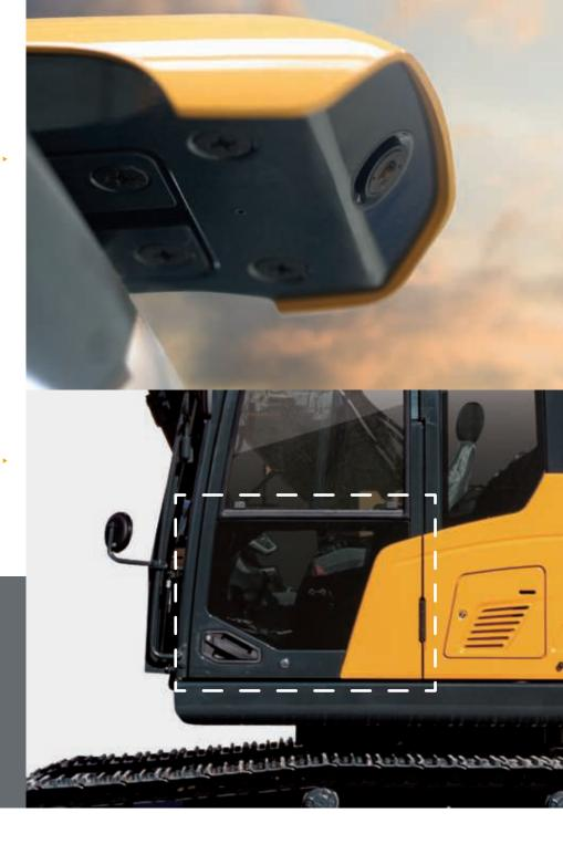
The **Advanced Around View Monitoring** (AAVM) camera system gives you a 360° overview of your immediate working environment. It also includes Intelligent Moving Object Detection (IMOD) technology that senses and warns you when people or objects come within five metres of the machine.
